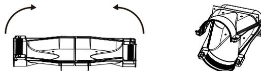
2. Rotate joint A and joint F into the two ends of heat discharge pipe. Then, rotate joint H to joint F, connect tightly
