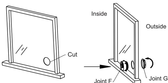
3. Install the other side of heat discharge pipe clockwise into joint F.
