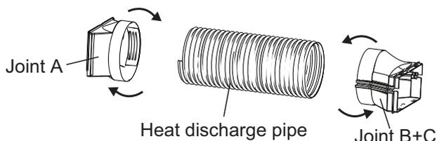
3. Insert joint A of heat discharge pipe (the side with "TOP" is upwards) into the groove until you hear a sound.
