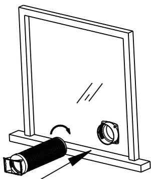
4. Insert joint A of heat discharge pipe (the side with "TOP" is upwards) into the groove until you hear a sound.
