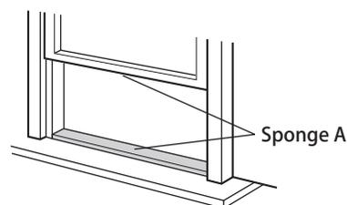
3. Attach the window panel to the window stool. Make sure that the exhaust cover is attached to the window panel.
