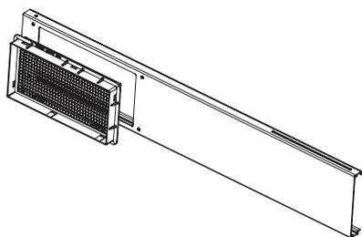
2. Cut the sponge A (adhesive type) to the proper length and attach it to the window stool and to the bottom of sash.
