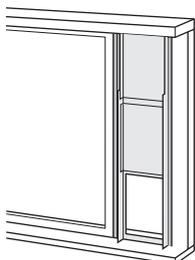
5. Stuff the foam seal B between the glass and the window to prevent air and insects from getting into the room.
