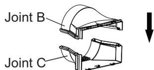
2. Rotate joint A and joint B+C into the two ends of heat discharge pipe.
