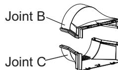
8. Rotate joint A and joint B+C into the two ends of heat discharge pipe.
